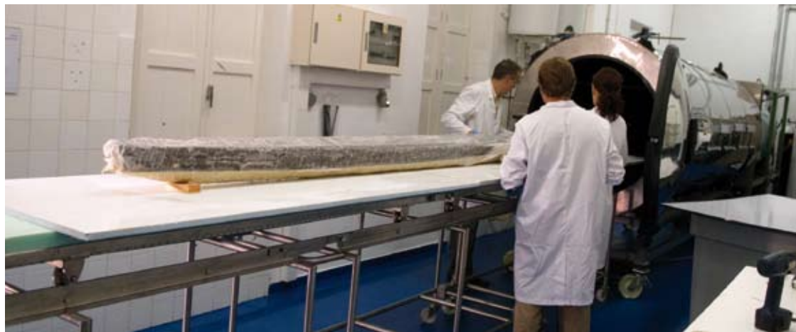
Wood laboratory. Freeze-dryer (ARQUA Archive, 2008).
